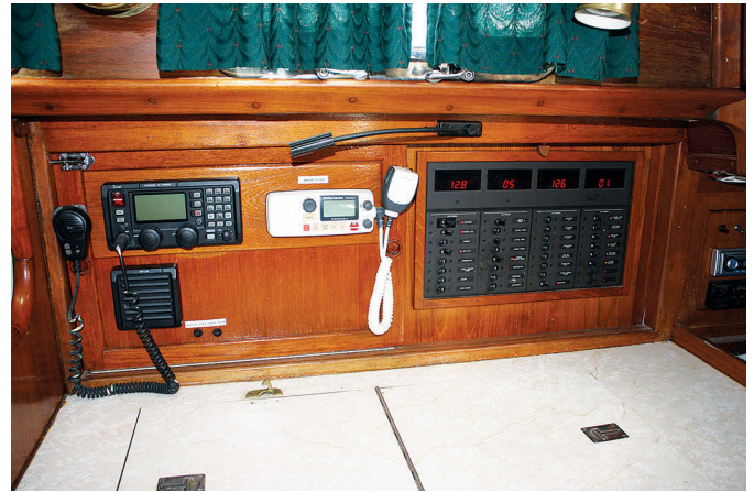
Gwyn works in the compact galley with Joshua, at left, who joined the crew as a rescue kitten soon after Ron and Gwyn bought Rapport . Refrigeration is on the starboard side. Ron built the new Bass electrical panel, at right, to replace the original panel, which was barely accessible and difficult to read. The side-by-side radios are an ICOM-M802 SSB (which receives GRIB weather data) and a West Marine VHF radio.
