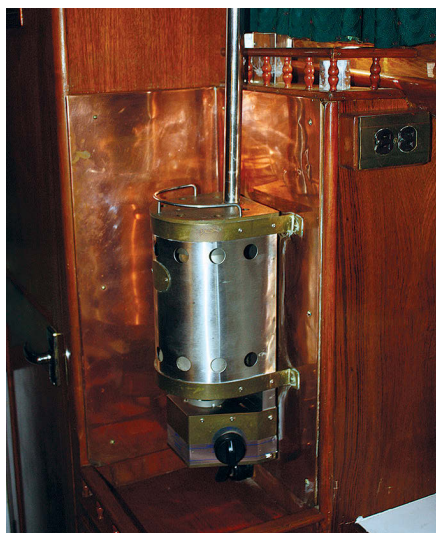
Originally a pilot berth, a large shelf area on the starboard side now holds the liveaboard home comforts of a microwave and an icemaker, at left. Just under the shelf, Ron built a narrow locker where they store paper charts flat. Ron also made the spice rack, at right. The Force 10 propane heater, below, is the right size to warm the cabin on chilly evenings at anchor.
